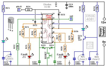
This is an enhanced 5 digit keypad which may be used with the Modular Alarm System.
