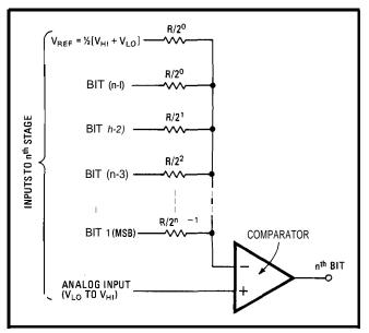
1. No stage. In n<sup>th</sup> stage of successive-approximation a-d converter, an analog input voltage that lies between  $V_{LO}$  and  $V_{HI}$  is compared with a voltage determined by an average of the reference voltage and weighted values of the more significant bits. Reference voltage Vref is fixed at the midpoint of the analog input range.
