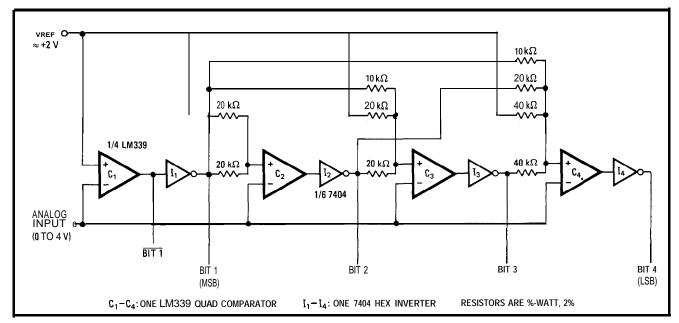
2. No **clock.** Comparator C, compares the analog input voltage with Vref. Thrs defines bit 1 and is averaged with Vref to set the switching level for C,. Bit 2 is averaged with both Vref and a weighted value of bit 1, to set the switching level for C3. Bit 4 is obtained similarly. Each output can drive one TTL load. LM339 comparators can sense input voltages down to ground potential, so only a + 5volt supply is needed.
