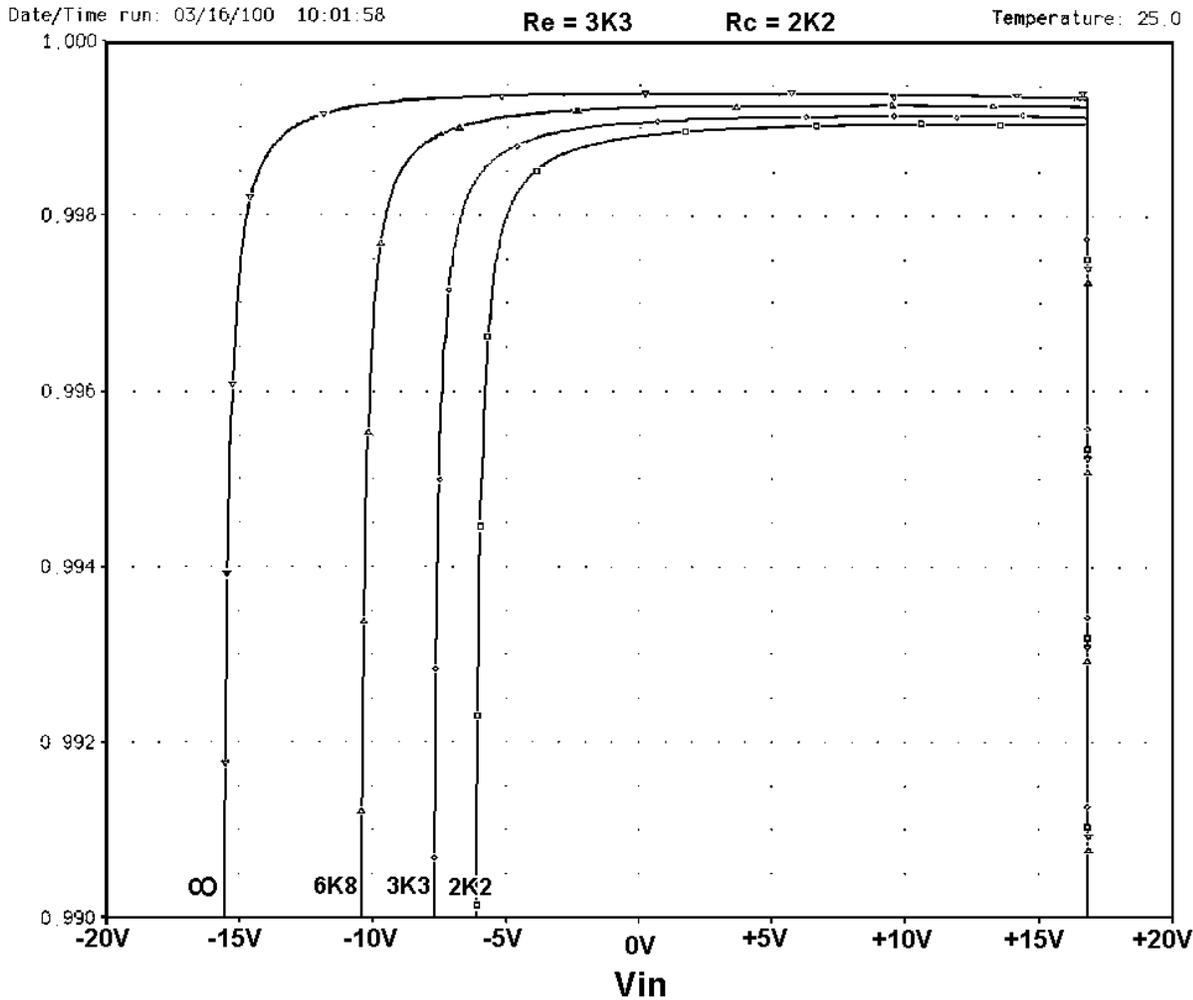
**Fig 10a: SPICE simulation of the circuit in Fig 9, for different load resistances.**
