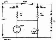
The circuit is built around the neon indicator which is normally used to show that power is being supplied to mains-driven equipment. When the fuse is intact, the neon is lit steadily as normal. However, should the fuse blow or be removed, the indicator flashes at a suitable rate, drawing the attention of the operator.
