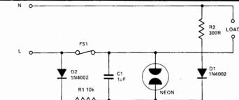
When the fuse blows, D2 blocks while
