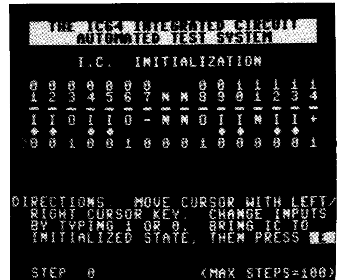
FIG. 6—THE FIRST TEST INITIALIZES each IC to a standard setup. The N shown for pin 11 indicates we don't care what the result will be on that particular pin.
