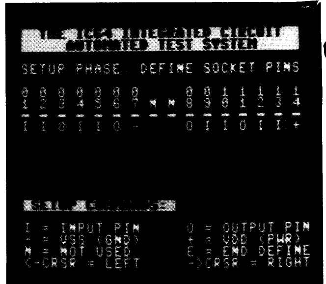
FIG. 5—FIRST STEP IN ANY TEST is to define the function of each socket pin, including the ground and +V connections.
