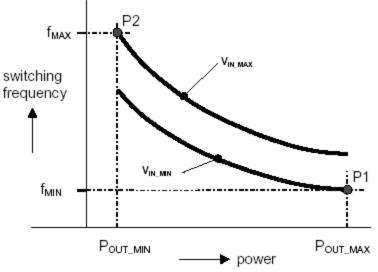
QR frequency characteristics at different input voltages
