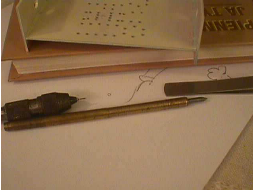
Picture 16: Two different bushing sleeve installation tools (Veikko Pöyhönen)
