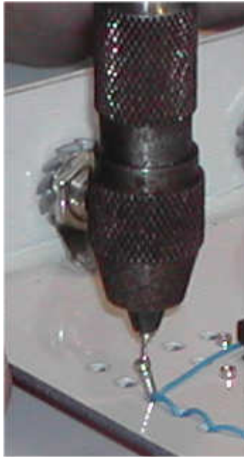
Picture 9: Sleeve installation tool mounted to a drilling (Tomi Engdahl)
